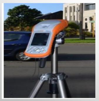
Quickly capture location and a calibrated image of any pole that allows for accurate measurement of attachments, heights and distances.
